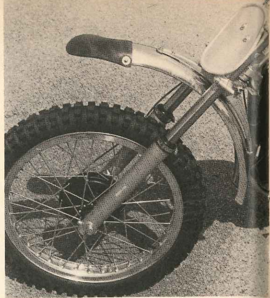
The front brake on the 400 Cross is slightly larger than on the 250. The difference in weight is not noticeable. Akront wheels are standard front and rear.
