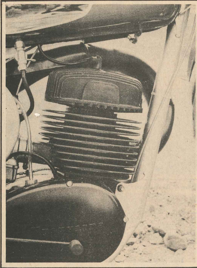
Massive fins aid in cooling a very "hot" machine.
