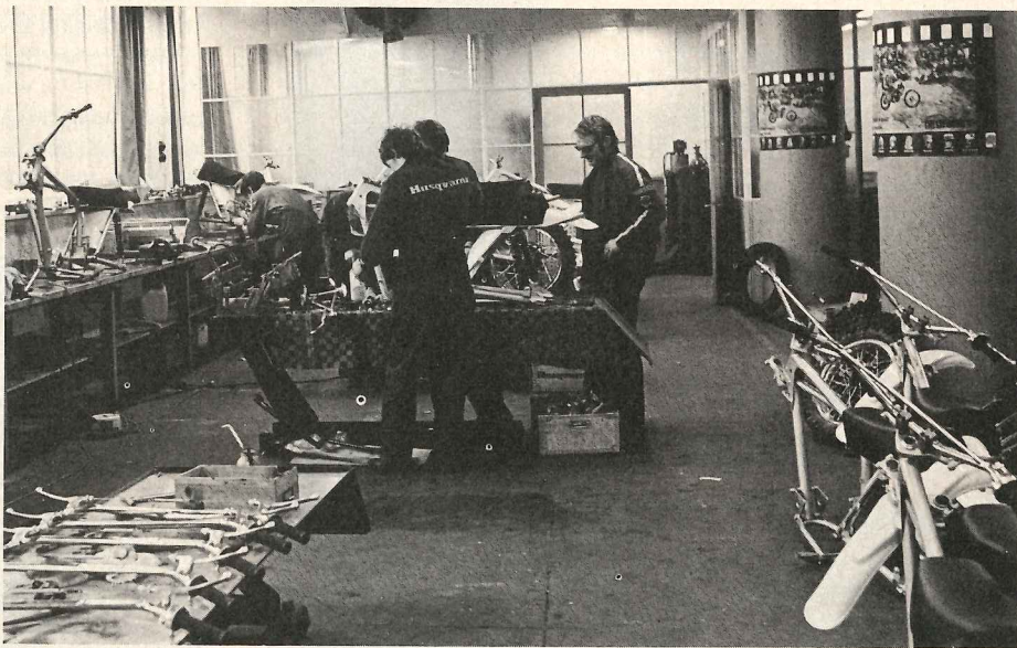
In the Husqvarna competition shop, 1973 "works" motocross machines are carefully assembled and checked.
