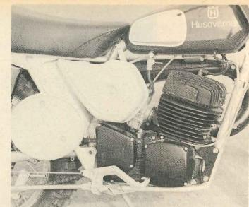
Behind the new air box lies a newer version of the 36mm Bing carb. Bike was easier to start. with only two prods to bring it to life.
