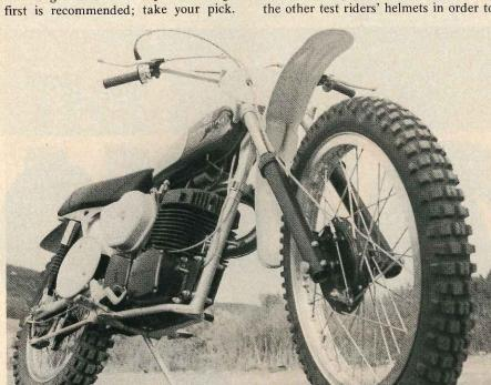
Magura levers, bent at a strange angle, make braking a pleasure. The pipe tucks well out of the way, and doesn't burn your leathers any more. Teflon cables enhance the bike, giving you more of the stock trickery.
