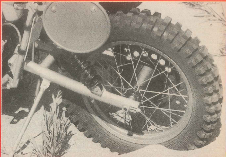
Chrome-moly swingarm and giant 5.00x17 Trelleborg rear tire. Shocks are wide body gas Girlings.
